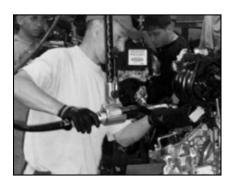
Carbon Arms and Carbon Torque tubes are simple, lightweight yet strong devices designed to absorb torque reactive forces. These innovative devices adapt to a wide range of tools and
