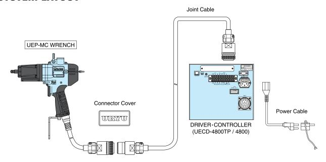
Uryu's unique feature, a non-contact and Magnetostrictive Transducer, provides tightening and fastening counter monitoring controlled by a highly accurate torque control mechanism connected to the multi-functional UECD-4800 Series controller (This is a combination unit of UEC-4800 and UEPD driver box).
