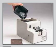
Load screws into the hopper.
