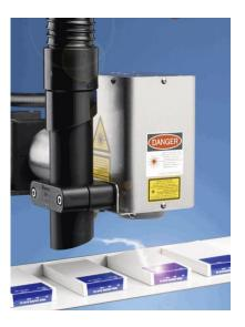
Uncaptured laser particulate will cause damage to optics, poor codes, beam divergence, sensor failure, handling equipment problems, fire hazards, respiratory hazards, and other problems.
