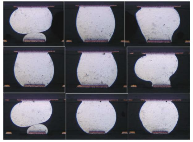
HIGH MAGNIFICATION OF OPEN CONNECTIONS SHOWING DISTINCT SEPARATION
