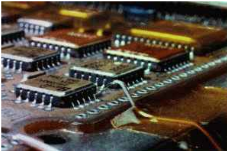
Figure 4: Tape Relaxed After Heating, Allowing The Thermocouple To Lift Off The Leg
