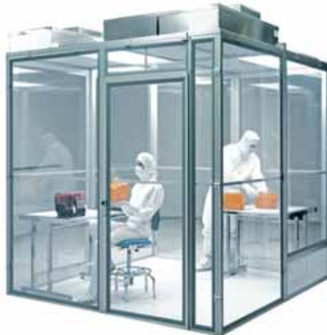
The concept behind a cleanroom is to push air into the room from the top, down into the room, and then out vents at floor level, carrying with it any contaminants from the manufacturing process. Note that these technicians are fully gowned.
