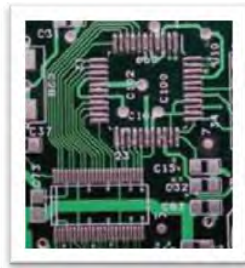
Figure 1. Circuit board with solder paste applied to pads
