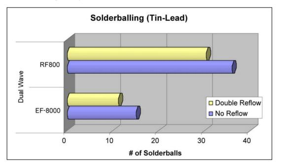
50% fewer solderballs observed on connectors processed with EF-8000 even after double reflow
