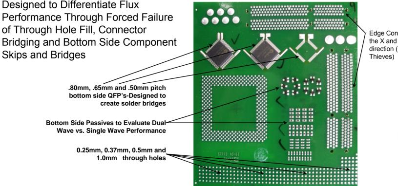
Edge Connectors in the X and Y direction (No Solder
