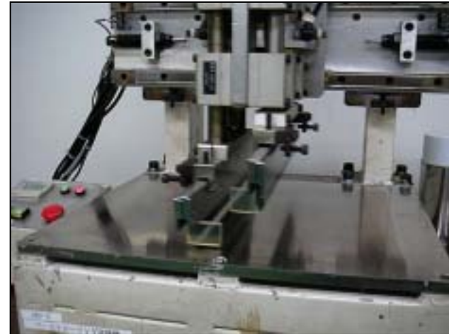
Custom Equipment simulating paste rolling on stencil with no replenishment
