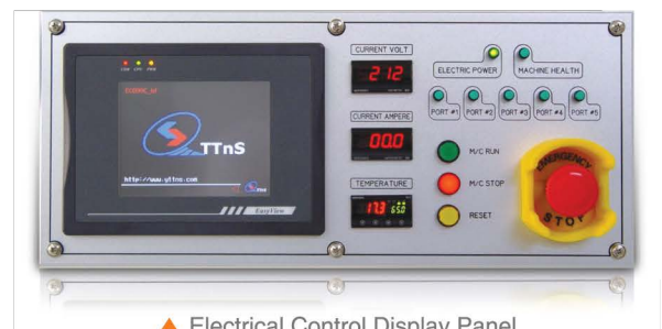
▲ Electrical Control Display Panel
