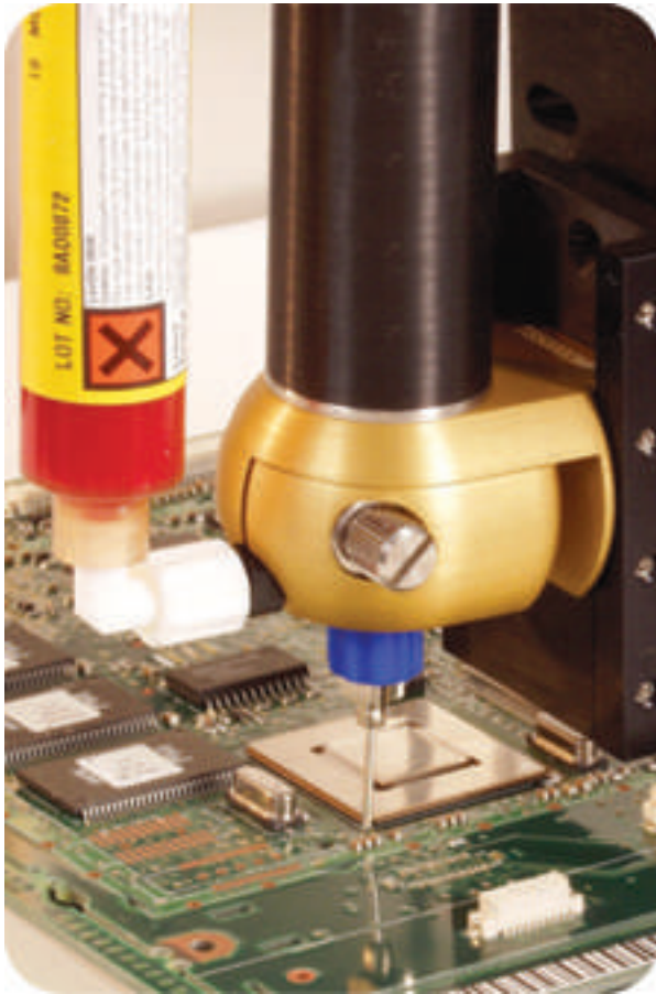
TS5000DMP - performing underfill.
