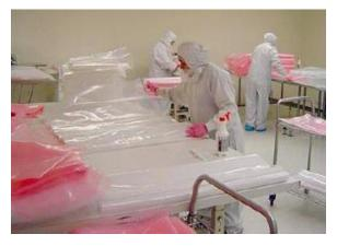
There are many different types of film and bags used in our industry. Low-density polyethylene (LDPE) virgin resin is the primary material of construction for cleanroom film. This material is available in many different thicknesses, widths, and lengths, and can be processed to meet special applications.
