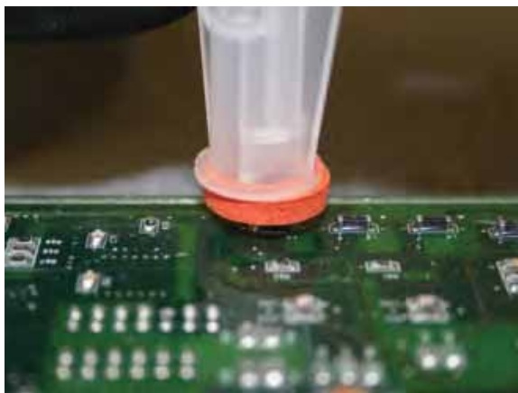
Localized extraction system seals over specific components.
