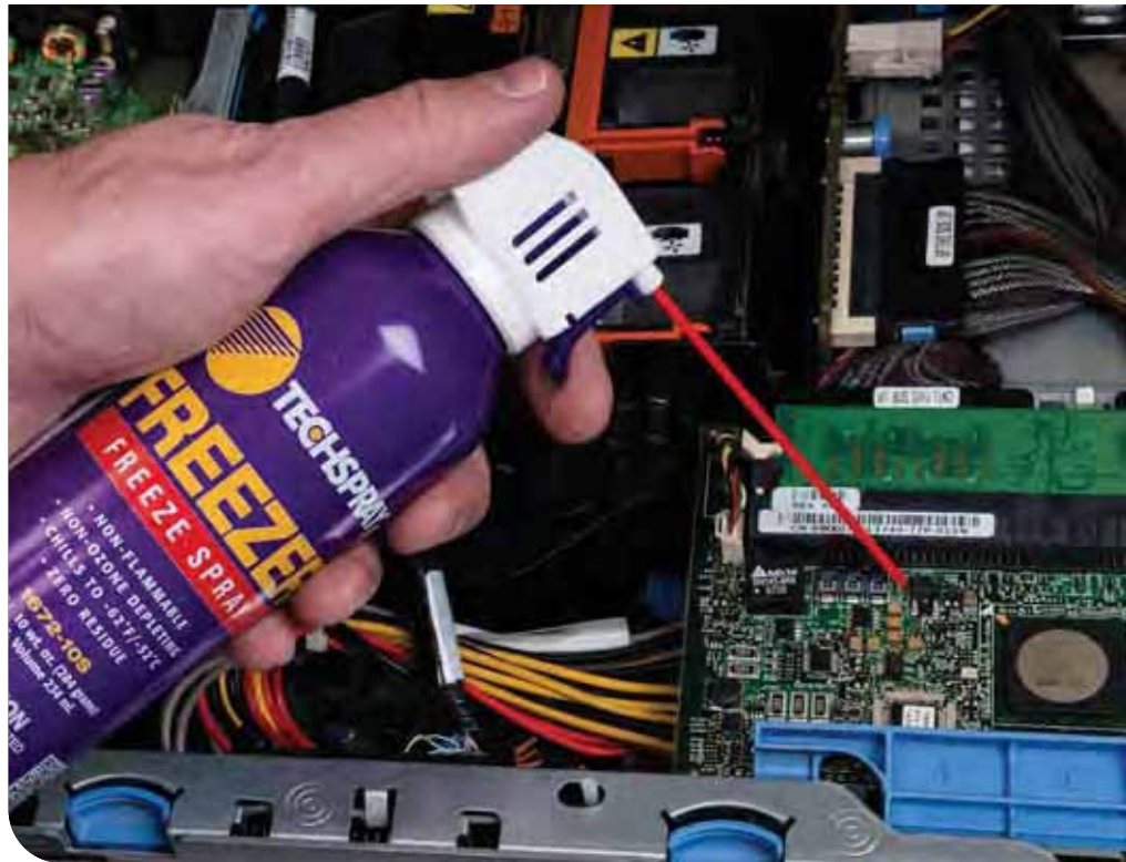
Freeze spray helps locate faulty components and cold solder joints.
