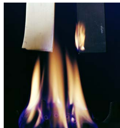
Flame resistance testing left: silicone rubber / right: organic rubber
