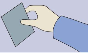
Clean the surface of all rust, oil, dirt, grime and other substances that may interfere with adhesion using sandpaper or a solvent (toluene, xylene, other). When cleaning plastics with solvents, use caution as some solvents may damage plastics.
