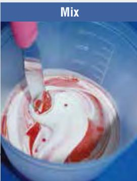
Combine the base polymer and curing agent, and mix until color is uniform and consistent.
