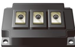
IGBT (Insulated Gate Bipolar Transistor) modules are a primary component of high-capacity inverters. In an IGBT module, a potting agent (gel) is used for electrical insulation and a sealant is used to bond the case to the base plate. In addition, a thermally conductive grease is used to help direct heat away from the IGBT module. For information on thermal interface greases, please see our Greases & Oil Compounds catalog.
