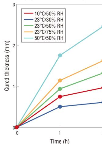
Effect of temperature & humidity on curing speed of KE-3495-W (7 days)
