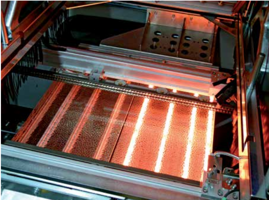
Figure 1. Full area bottom-side IR preheat module with emitters switchable to match preheat requirements.
