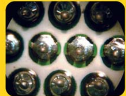
Solder paste and preforms reflowed
