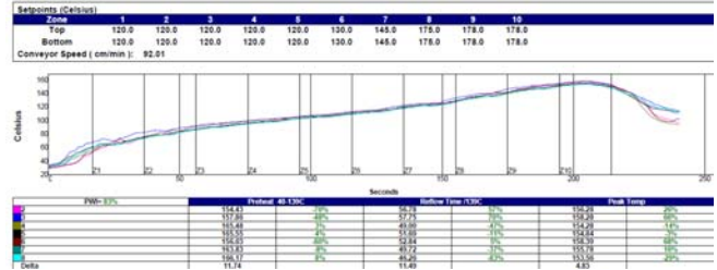
Figure 6 Low Temperature Reflow Profile
