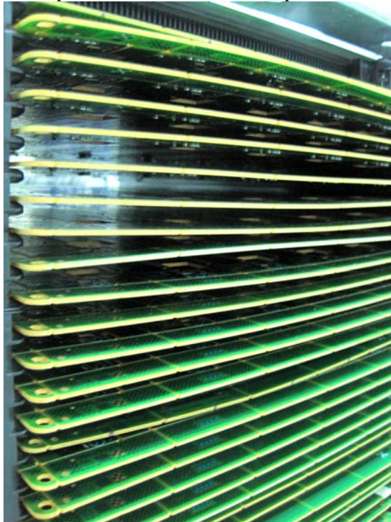
Figure 7-Warped FR-1 Boards after SAC Reflow Profile
