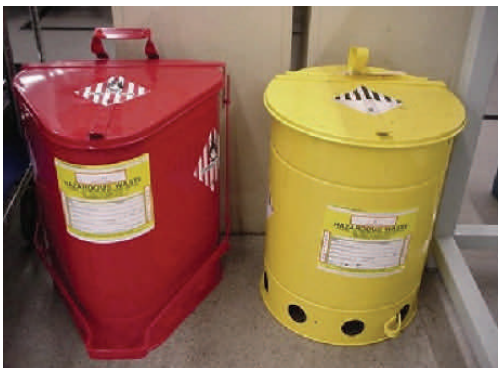
Figure 2. Hazardous waste containers.
