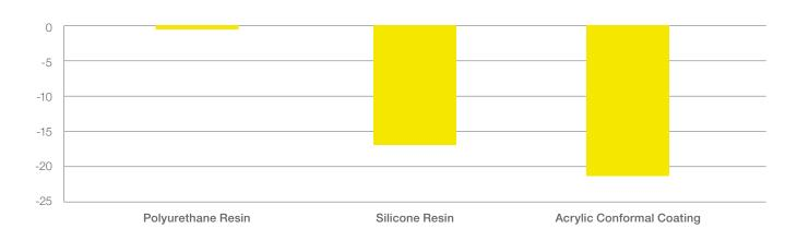
When considering the protection and performance of electrical switches and contacts, it is also important to consider the performance in humid or corrosive environments. In order to establish which products provide the highest level of protection in high humidity and corrosive environments; test panels were coated with Electrolube Contact Lubricant products and subject to 90%RH, 35°C for 3 weeks, followed by 1 week in the salt spray chamber using a 5% salt solution.
