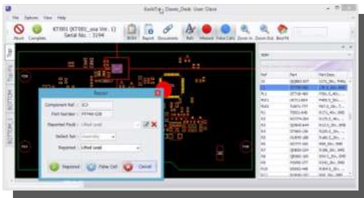
Defect validation page comparing defect reported to defect found, location on PCB, part number, description, reference designator
