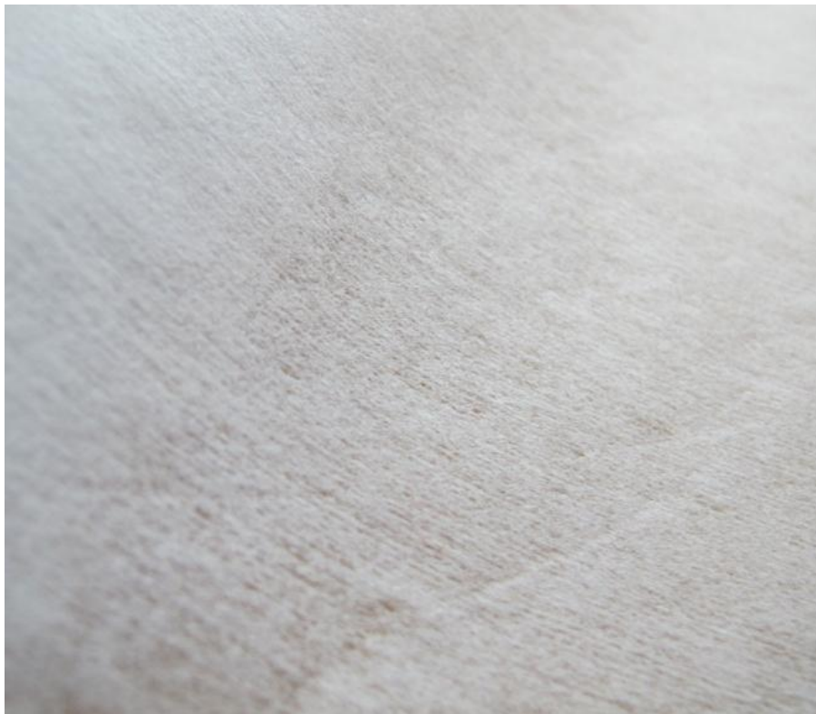
Figure 8 – Photo of cleaning paper C. Even surface, darker “lines” with less material.
