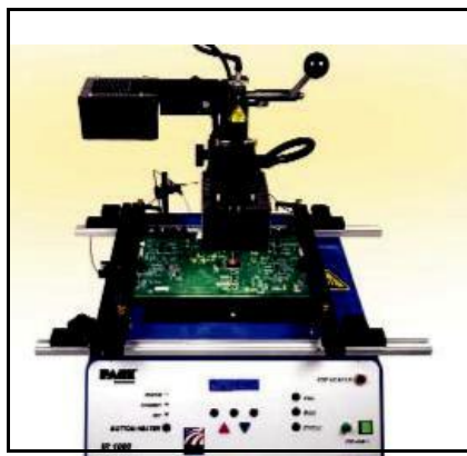
Standard BGA system using IR Preheat.
